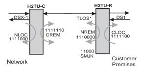
\* When enabled, TLOS is an automatic loopback that occurs with an LOS at the remote DS1 input.
