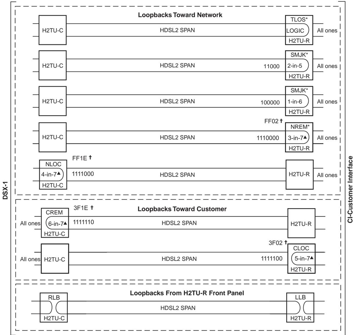
\* Set the NLBP option to AIS to send AIS (indicated by an all ones pattern) for any network loopback.
