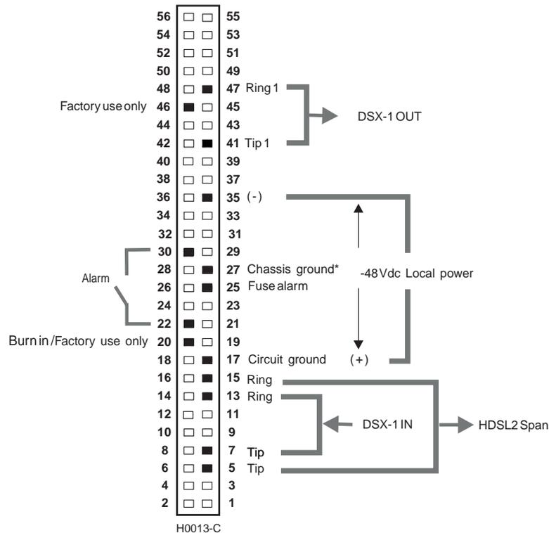
\* Chassis ground may be connected to Earth ground per local practice.
