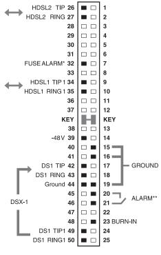
\* Fuse alarm is normally floating and at -48V when activated.
