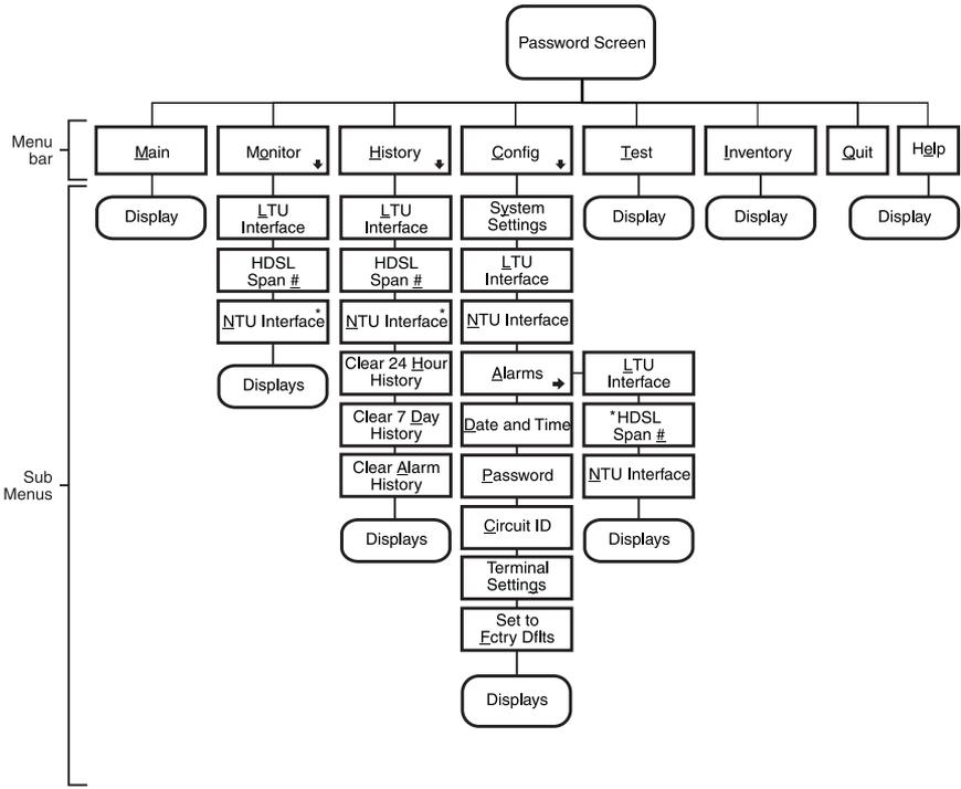
**Figure 8.** Console Screen Menu Structure
