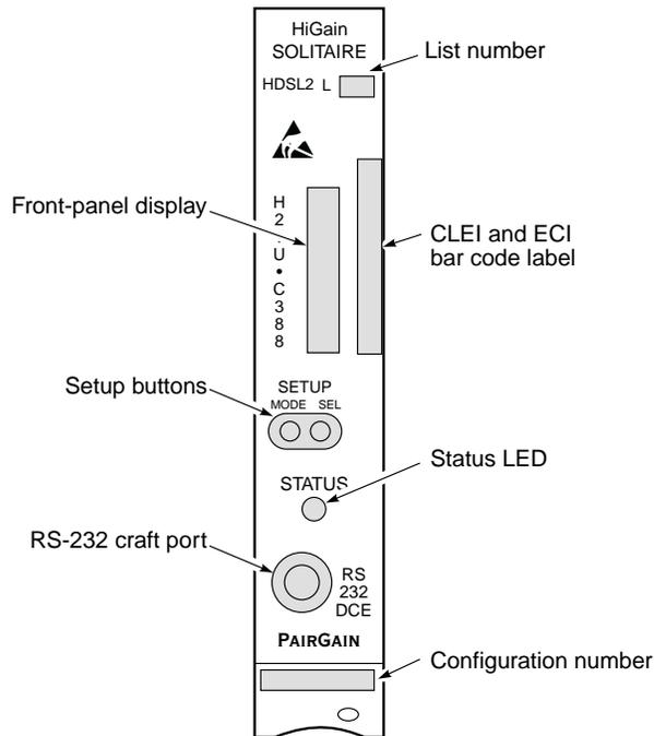
Figure 2. H2TU-C-388 List 1E Front Panel
