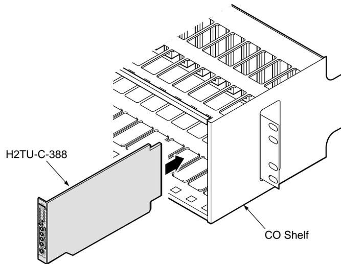
*Figure 3. Installing the H2TU-C 388 List 1E into a Shelf*
