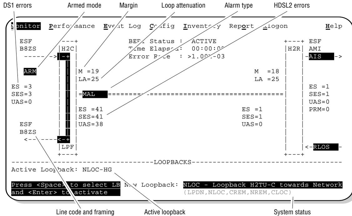
Figure 12. Monitor Screen - Active Loopback with Alarms
