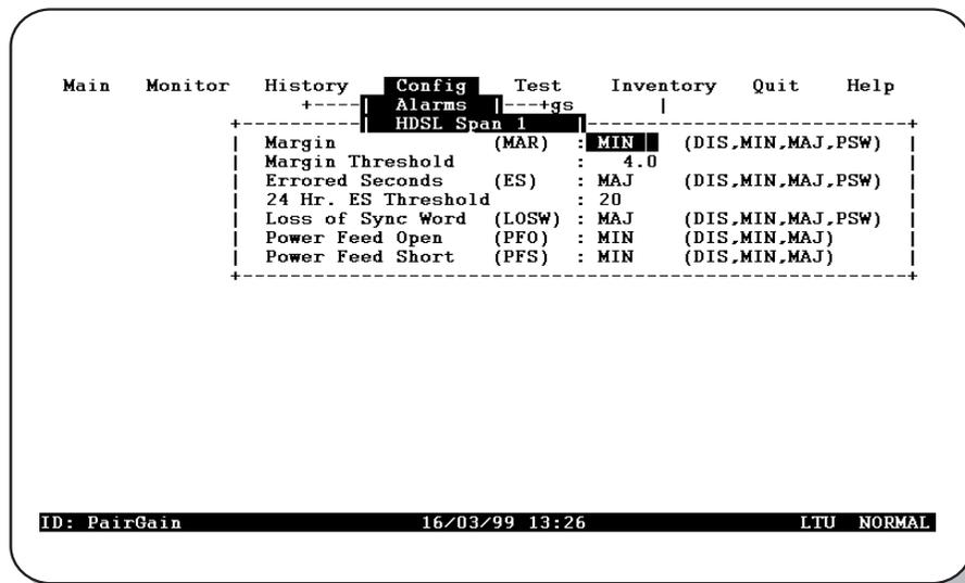
**Figure 29.** Config Alarms HDSL Span 1 Menu
