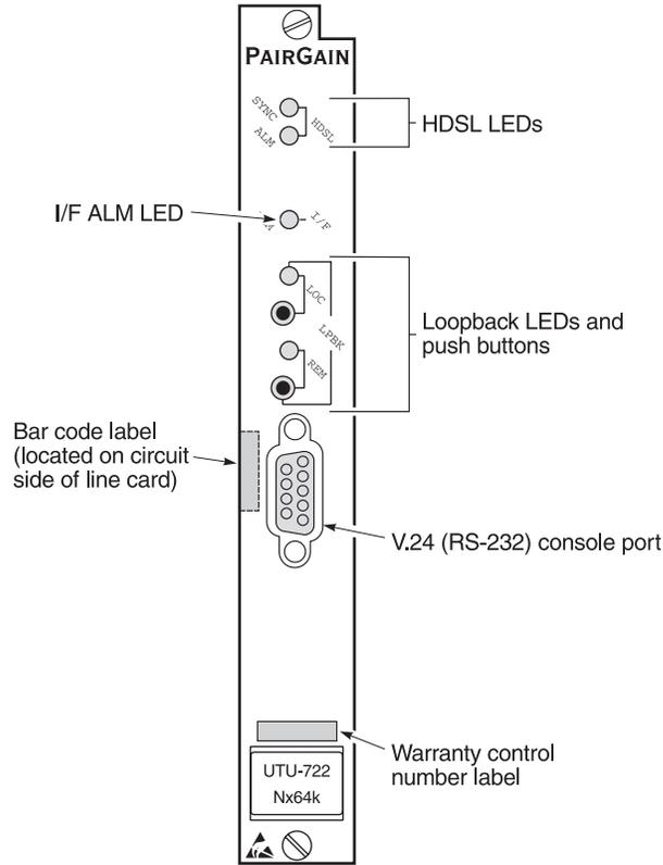
**Figure 2.** UTU-722 Line Unit Front Panel
