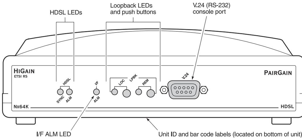
**Figure 3.** ETU-772 Desktop Unit Front Panel
