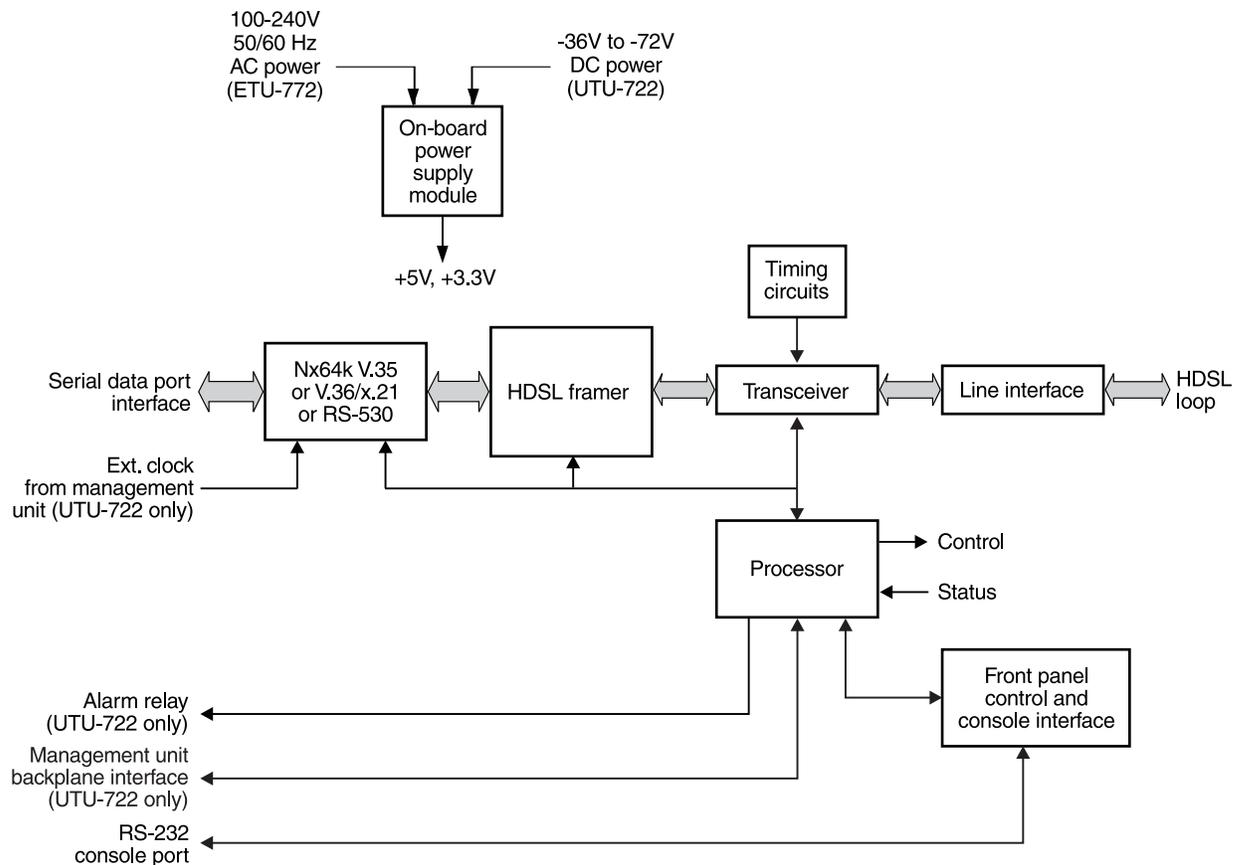
Figure 5. Line and Desktop Unit Functional Block Diagram
