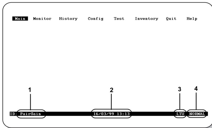
**Figure 17.** Items in Console Screen Status Bar
