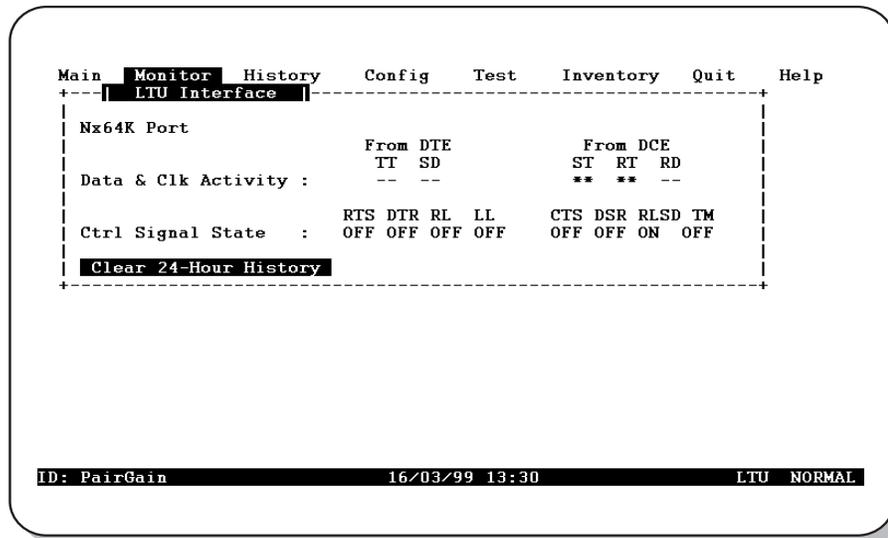
Figure 33. Monitor LTU Interface Screen
