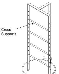
3 The pedestal framework is now ready for installation of the FRE-860 RT Enclosure.
