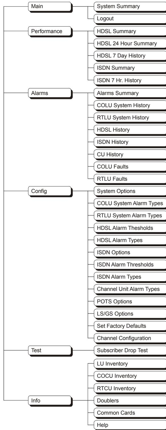
Figure 7. Terminal Menu and Display Structure (Universal)
