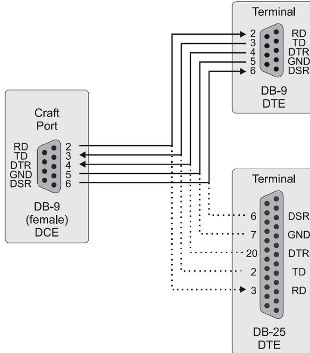
**Figure 5. Front Panel Craft Port to Terminal Connections**
