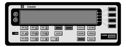
For Maxwell Technology Series 4000 GPS receivers with the EVEREST firmware option installed (for example, the 4000SSE, 4000SE System Surveyor II and 4000SSi), the postprocessed differentially corrected accuracy (CEP) is specified as 50 cm +1 ppm, subject to the following conditions: at least five satellites, PDOP less than four, a Base station with the EVEREST firmware installed, and a baseline length of less than 1,000 km.
