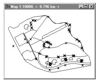
You can define what elements you want to view on this screen, and you can display positions and features simultaneously or separately by selecting or de-selecting the appropriate check boxes in the dialogs displayed using the *View / Layers* command.
