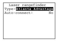
Set the *Type* field to *Atlanta Advantage*. If you will generally be using the Advantage rangefinder when capturing data, and if you will typically *not* be using any other type of external sensor, then set the *Auto-connect* field to Yes.
