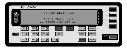
To clear these messages, press the  $\boxed{CLEAR}$  button on the 4000's front panel.
