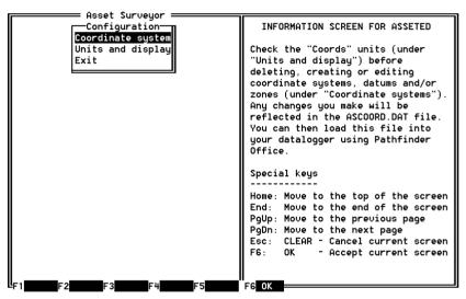
The ASSETED program has a user interface which is similar to that of the Asset Surveyor software, so you should find it reasonably familiar. The panel to the right of the PC's screen provides information about special keys. The most important keys to remember are the  $\boxed{ESC}$  key (which acts like the  $\boxed{Clear}$  key on the TDC1) and the  $\boxed{OK}$  softkey (which acts like  $\boxed{OK}$  on the TDC1).
