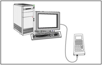
Figure 3-3 Direct Connection between TDC1 and PC
