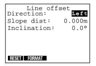
A line, area or quickmark offset can also be displayed and entered as a horizontal distance, a vertical distance (above the horizontal) and a direction:
