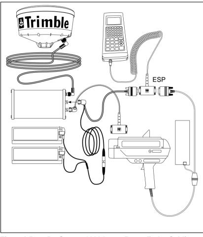
Figure I-5 ProSurvey 1000 Laser Rangefinder Cabling Diagram for Pro XR with TDC1
