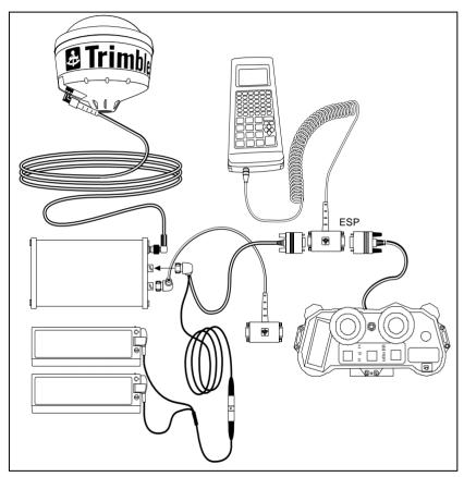
Figure I-10 Ledha-Geo Laser Binoculars Cabling Diagram for Pro XRS with TDC1
