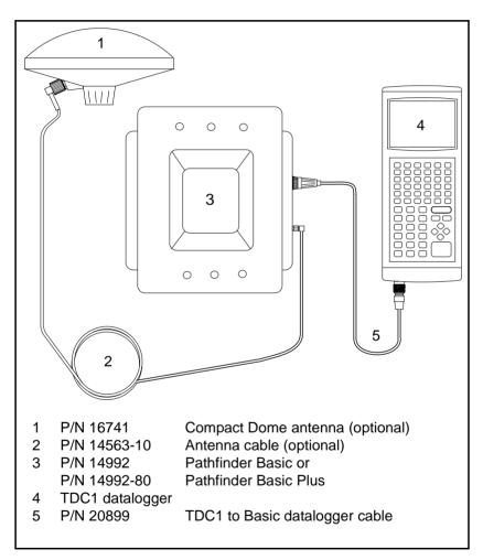
Figure D-2 Cabling for the Pathfinder Basic
