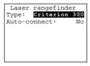
Set the *Type* field to either Criterion 300 or Criterion 400. If you will generally be using a Criterion rangefinder when capturing data, and if you will typically *not* be using any other type of external sensor, then set the *Auto-connect* field to Yes.
