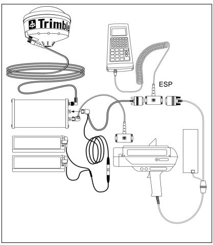
Figure I-4 ProSurvey 1000 Laser Rangefinder Cabling Diagram for Pro XRS with TDC1
