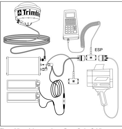
Figure I-7 Advantage Laser Rangefinder Cabling Diagram for Pro XRS with TDC1
