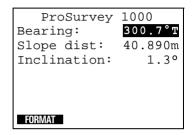
Asset Surveyor displays the distance measurement in the currently configured *Distance* units. The laser azimuth (bearing) is converted to a true North azimuth. If the configured *North ref* is *True*, it is immediately displayed as a true North bearing (with a 'T' suffix); otherwise it is displayed as a magnetic North bearing (with a 'M' suffix).
