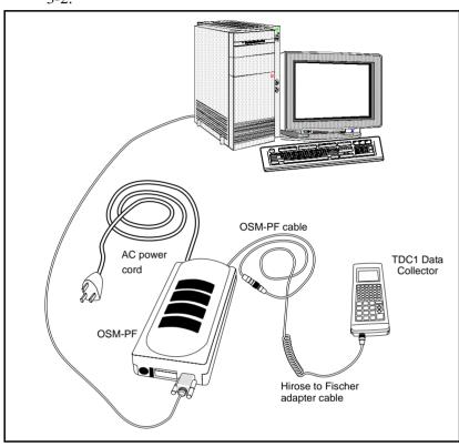
3. Plug the OSM-PF AC power cord into an AC outlet. See Figure 3-2.
