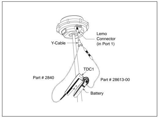
Figure G-3 4600LS Surveyor Mounted on Range Pole with TDC1 Asset Surveyor, Y-Cable, and Camcorder Battery
