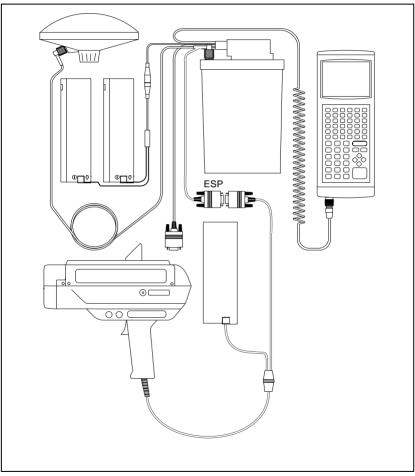
Figure I-6 ProSurvey 1000 Laser Rangefinder Cabling Diagram for Pro XL with TDC1
