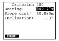
Asset Surveyor displays the distance measurement in the currently configured *Distance* units. The magnetic laser azimuth (bearing) is converted to a true North azimuth. If the configured *North ref* is *True*, it is immediately displayed as a true North bearing (with a 'T' suffix); otherwise it is displayed as a magnetic North bearing (with a 'M' suffix).
