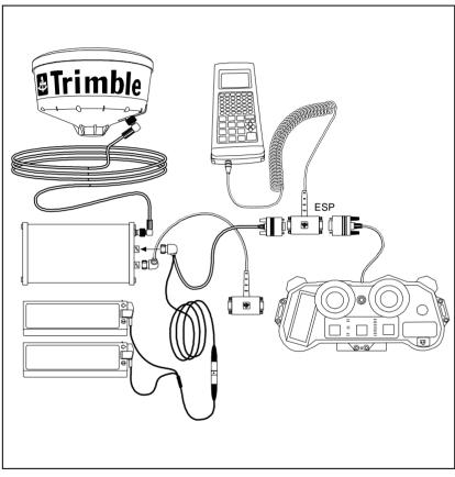
Figure I-11 Ledha-Geo Laser Binoculars Cabling Diagram for Pro XR with TDC1
