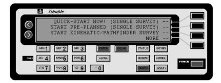
Press the <u>CLEAR</u> button to avoid starting a survey logging in the memory of the Series 4000 receiver and proceed to the receiver's main status screen:
