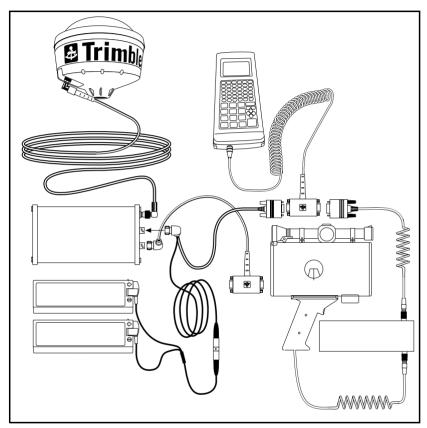
Figure I-1 Criterion Laser Rangefinder Cabling Diagram for Pro XRS with TDC1
