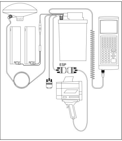
Figure I-9 Advantage Laser Rangefinder Cabling Diagram for Pro XL with TDC1
