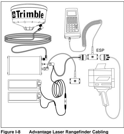
Jure I-8 Advantage Laser Rangefinder Cabling Diagram for Pro XR with TDC1
