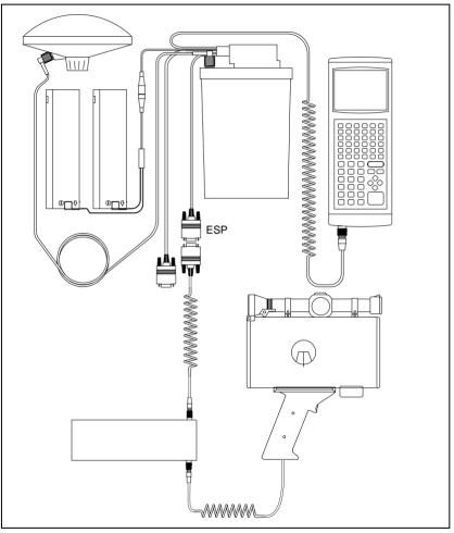
Figure I-3 Criterion Laser Rangefinder Cabling Diagram for Pro XL with TDC1
