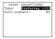
Set the *Type* field to *ProSurvey 1000*. If you will generally be using the ProSurvey 1000 rangefinder when capturing data, and if you will typically *not* be using any other type of external sensor, then set the *Auto-connect* field to Yes.
