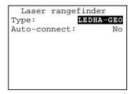
Set the *Type* field to *LEDHA-GEO*. If you will generally be using the Ledha-Geo laser binoculars when capturing data, and if you will typically *not* be using any other type of external sensor, then set the *Auto-connect* field to Yes.
