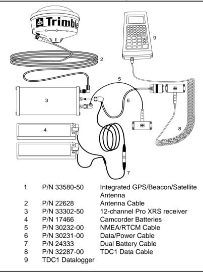
Figure A-1 Cabling for the Pathfinder Pro XRS
