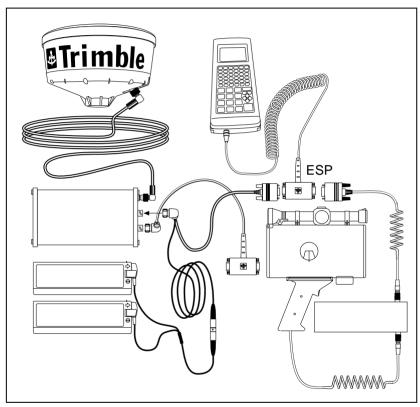
Figure I-2 Criterion Laser Rangefinder Cabling Diagram for Pro XR with TDC1
