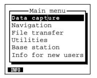
From this menu, you can choose one of the five main Asset Surveyor operations. The sixth entry in the menu (*Info for new users*, which you can also access using **DIFO**) provides access to several pages of information for new users of the software. You can configure the Asset Surveyor software by pressing *Config.* The Asset Surveyor software's *Configuration* menu is as follows:
