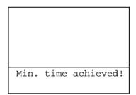
You have logged sufficient carrier phase data to achieve the precision required for the features captured since the counter was last reset, and until it is again reset.
