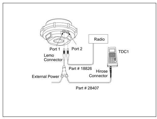
Figure G-4 4600LS Surveyor RTCM Input Configuration with Radio, TDC1 Asset Surveyor, and External Power
