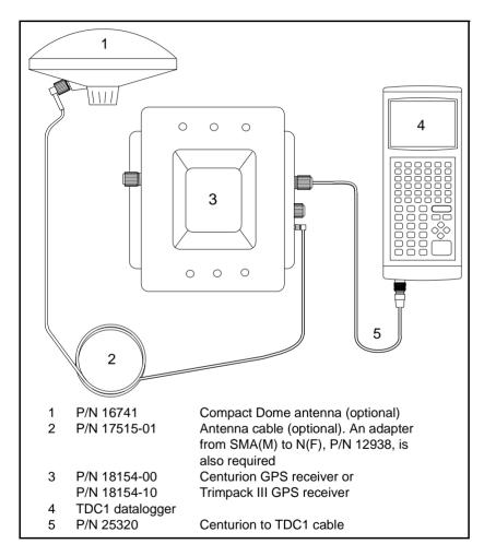
Figure E-1 Cabling for the Centurion or Trimpack III
