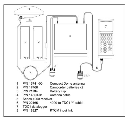
Figure F-1 Cabling for the Series 4000 Receiver
