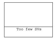
because the GPS receiver is tracking fewer satellites (probably none) than it needs to compute positions.
