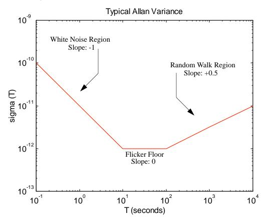
The downward slope represents the area of white noise. Lower is better. Notice that the line decreases with time. An intuitive way to think about the Allan Variance is to think of the distance from the X-axis to the line as the slope of a line that can be drawn through a section of oscillator performance.
