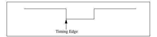
Figure 5-8 10 MHz with positive zero crossing (shown with rising edge)
