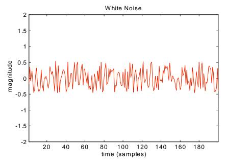
As time passes, errors begin to add up and the oscillator starts to drift from truth. This drift becomes more dramatic over longer periods. Mathematically the nature of the oscillator performance changes. White noise has a statistical average or mean that is zero. Over longer periods the oscillator's mean is constantly changing. This creates a "random walk" pattern.
