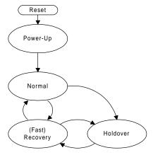
In the Normal state, the ThunderBolt maintains the synchronization of the timing outputs using phase-locking. As long as valid GPS signals and measurements are received, the ThunderBolt is as happy as can be. Any disruption in the GPS receiver (e.g. loss of GPS
