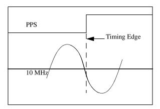
The PPS is generated from the 10 MHz and the rising edge will match the zero crossing within 10 nanoseconds. When the PPS is adjusted using the cable delay command, the phase of the 10 MHz will move by the same amount so that the rising edge of the PPS always corresponds to the zero crossing of the 10 MHz.
