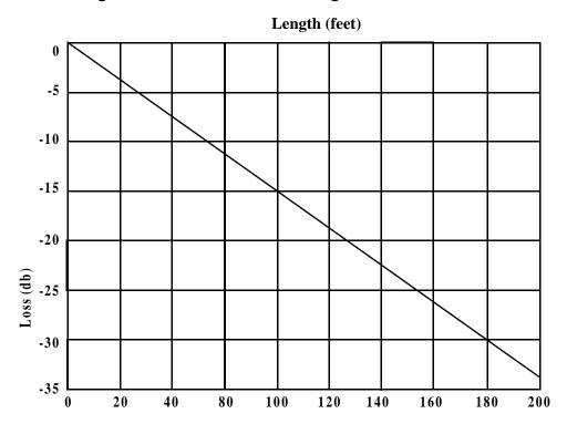
Figure 3-6 RG-8: Loss vs. Length
