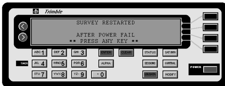
To clear these messages, press the **CLEAR** button on the 4000's front panel.
