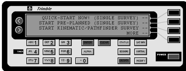
Press the **CLEAR** button to avoid starting a survey logging in the memory of the Series 4000 receiver and proceed to the receiver's main status screen:
