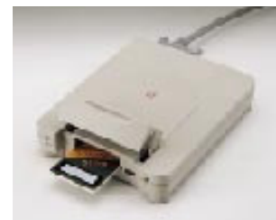
An external PCMCIA card drive, such as the Card Pro or Databook TMD-650, can be attached to your desktop computer.
