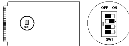
Figure 1-20. Tone Receiver Card DIP Switch
