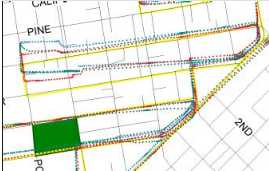
Figure 5: Position error due to change in elevation. Dotted lines are position tracks from 3 different tests on the same steep hill in San Francisco.
